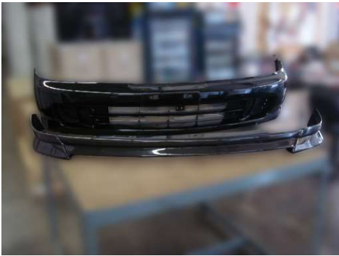
Fig. 1 Remove the bumper and place lip onto the bumper. Do not force the lip onto the bumper. Pay attention to the fitment to figure out what modification will be needed for installation.
