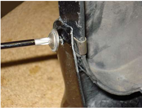
Fig. 7 Install the screws but don't completely tighten them yet. Leave room for adjustments if needed.
