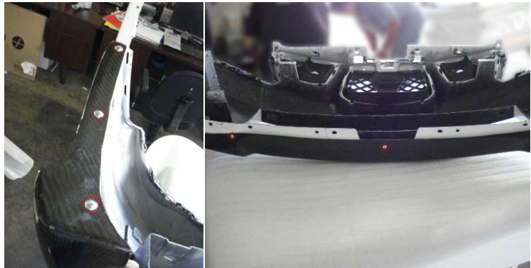
Fig. 8 Use previous steps in fig. 6 and 7 to complete installation. Once all screws are in place, finish your installation by tightening all the screws.
